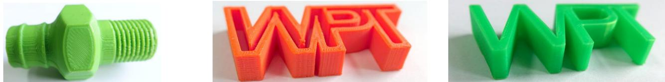
Fig. 1. 3D models made of PLA and ABS filaments
