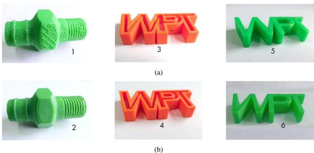
Fig. 3. Models printed at ambient temperature (a), models printed in the heated chamber
